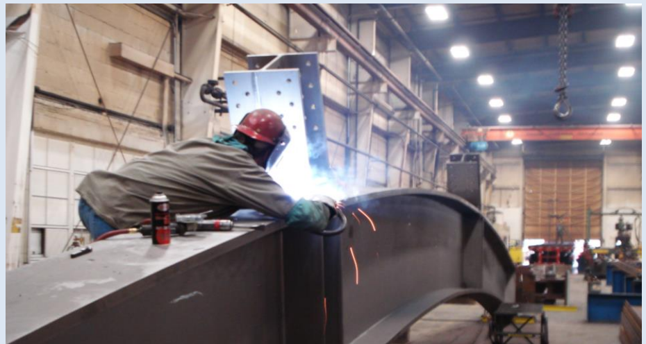
High Steel Structures, LLC fabricates enormous steel girders for the New NY Bridge project.
